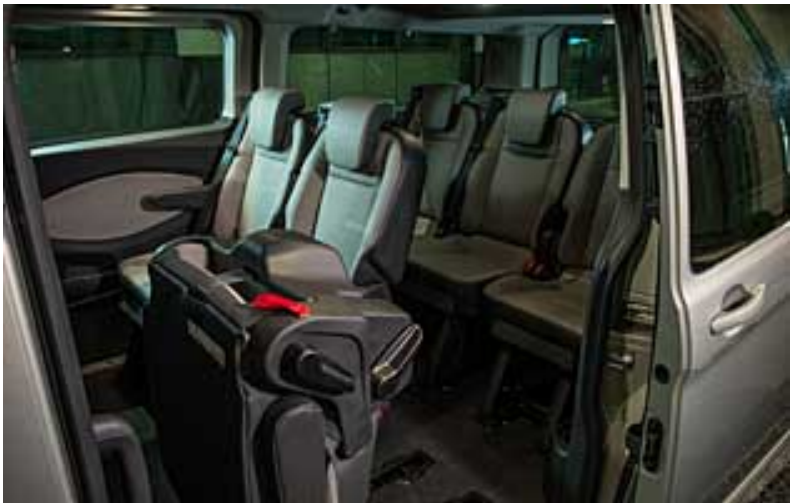
Vehicle with three rear seats. Seat required to move forward before a passenger can enter or egress the back seats
